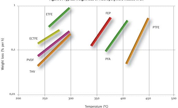
Figure 1: Typical weight loss of Fluoropolymers heated in air
